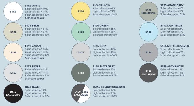
\*Please consider on south-facing elevations the high solar heat gain during the summer months may result in the glass being too warm to touch. In this case, we recommend a high solar control glass type such as SKN 176 which will reduce but not eradicate the heat. Please bare this in mind when choosing the colour of your Uni-Blinds<sup>®</sup> especially S158, S159 and B160.
